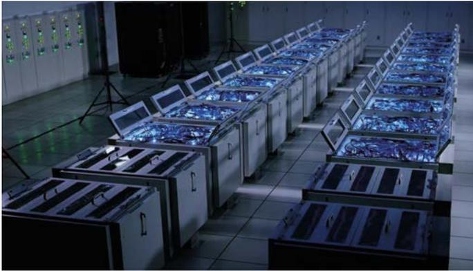
**Figure 4: The liquid-cooled Gyoukou ExaScaler/PEZY ZettaScaler-2.2 supercomputer**
